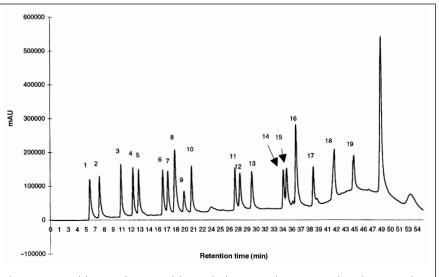
**Figure 1.** HPLC of the PITC derivative of the standard amino acids: aspartic acid, 1; glutamic acid, 2; hydroxy-proline, 3; serine, 4; glycine, 5; threonine, 6; alanine, 7; histidine, 8; proline, 9; arginine, 10; tyrosine, 11; valine, 12; methionine, 13; isoleucine, 14; leucine, 15; norleucine (internal standard), 16; phenylalanine, 17; tryptophan, 18; and lysine, 19.
